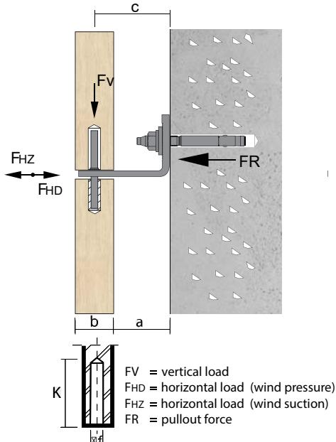
MATERIALS SS304, SS316, SS31L, SS316Ti, S235JR-MG, S235JR-HDG 50°C 24H average temperature standard items:
